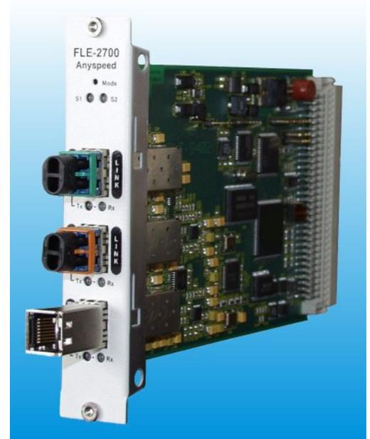
The new FLE-2700 card works with the “Anyspeed” technology. This means, that the FLE-2700 supports any transfer rate from 0,1 to 2,7 Gbps. On this reason any common application from Fast Ethernet to STM-16 can be transferred with one single FLE-Card.
